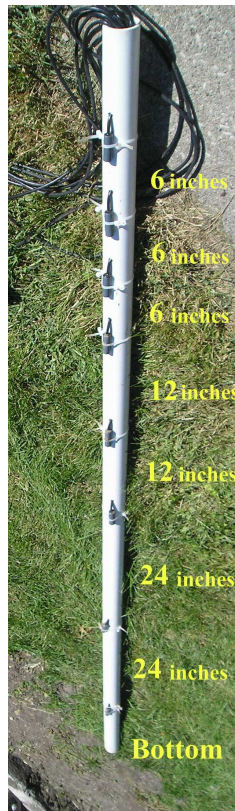
Figure 170 -- Temperature sensors mounted on the PVC pipe.
