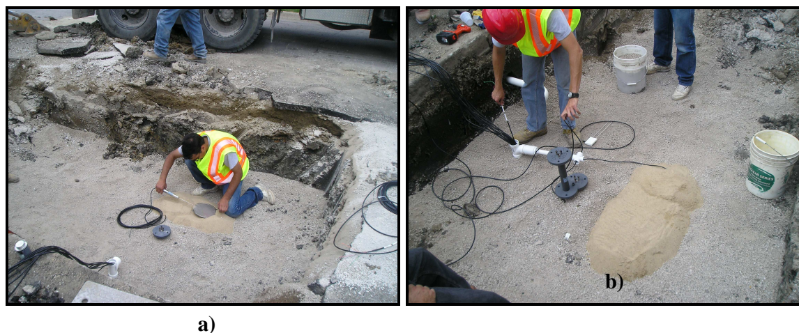
Figure 167 -- Pressure cell being placed within a lens of sand, a) sand lens below the pressure cell and b) sand lens covering the pressure cells
