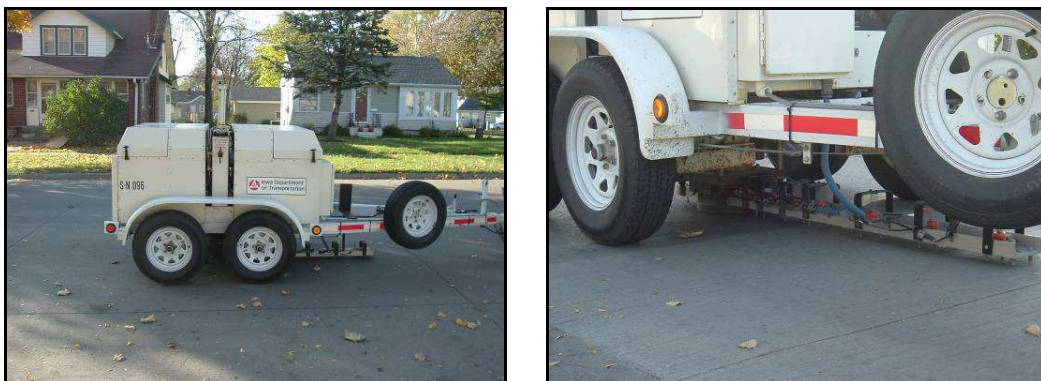
Figure 9 -- Iowa DOT FWD equipment
